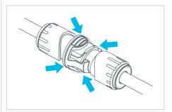
Firmly push the opposing ends of connector together, until latched, activating internal gas blocking mechanism.
