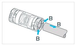
B – Push the collet down into the connector and pull the microduct away.
