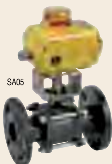
765 XS - Electric actuated carbon steel ball valve A216WCB body - CF8M ball - TS: -25°C/+220°C - ⚠ Steam use: PS: 15 bar / TS: +200°C.
