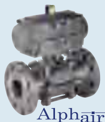
711 XS - Pneumatic actuated stainless steel ball valve Direct mounting - CF8M body & ball - TS: -30°C/+218°C.
