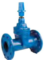
184 - EPDM wedge - EN 558 series 15 (DIN 3202 F5) - With square drive nut ⌚
